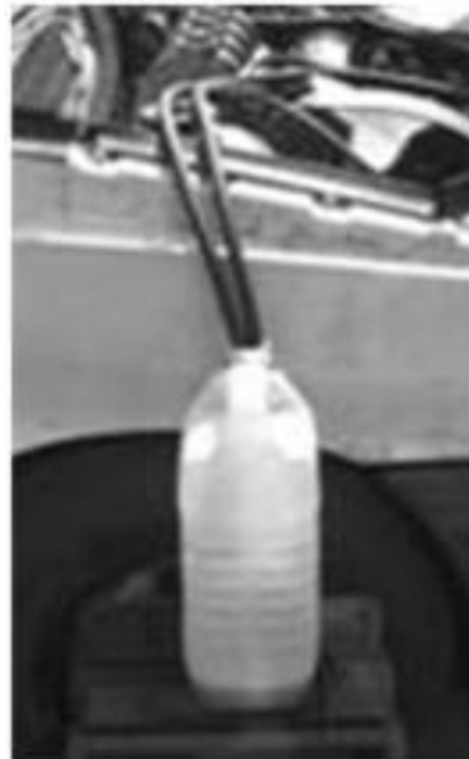
Fig. 1 External tank and of the fuelling lines
